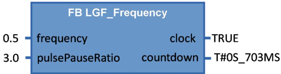
$$pulsePauseRatio = \frac{t_{on}}{t_{off}} = \frac{3}{1}$$
